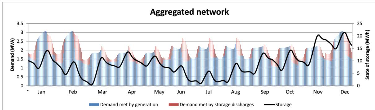
**Figure 4** Combined generation and aggregated storage
