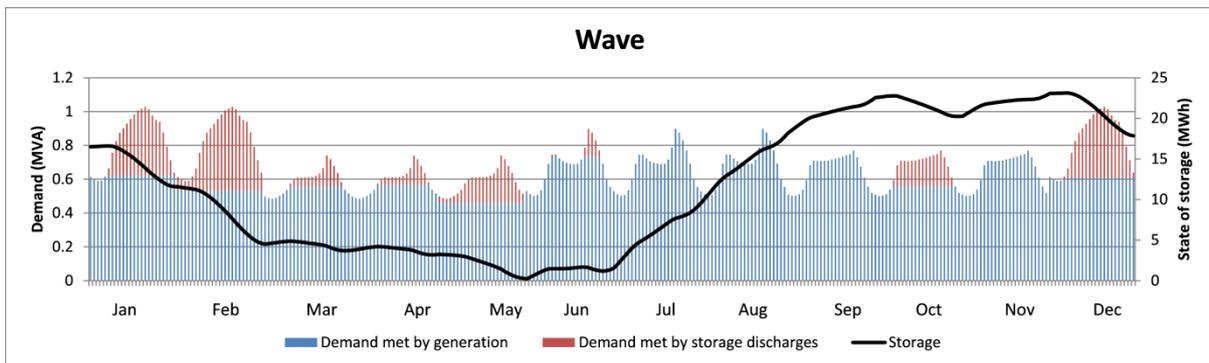
**Figure 4** Wave generation and energy storage
