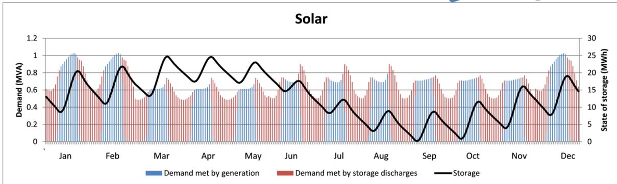
**Figure 2** Solar generation and energy storage
